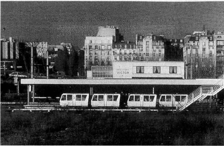
11. Aramis really does exist now; here it is in 1987, pulling up to the experimental station on the boulevard Victor. Each pair is made up of two ten-passenger cars, coupled mechanically like standard train cars; but the only connection between pairs is the electronically calculated “nonmaterial coupling.” [Photo Matra]
