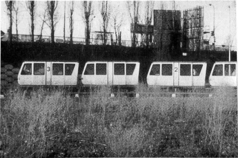
12. The nonmaterial coupling allows passengers who are heading for two different destinations to get on at the same station. When they leave the station, the two pairs of cars proceed together, adjusting the distance between them through the principle of the CMD (adjustable mobile sector) like cars in a lane. [Photo RATP]
