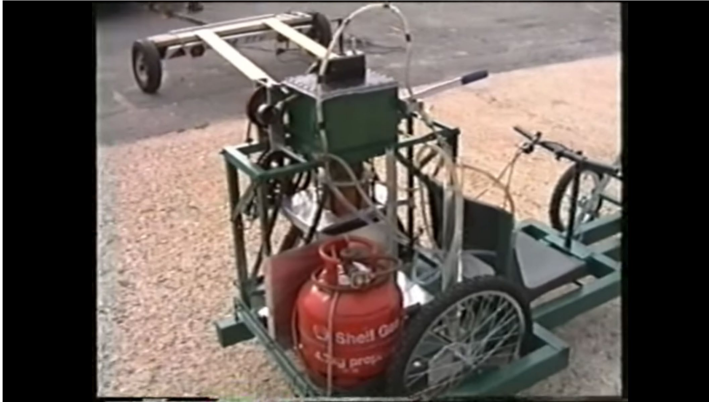
Road testing a Stirling engine powered buggy, (filmed in Norwich England, 2001)
